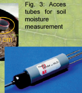
Fig. 4: FD-Probe for soil moisture measurement
