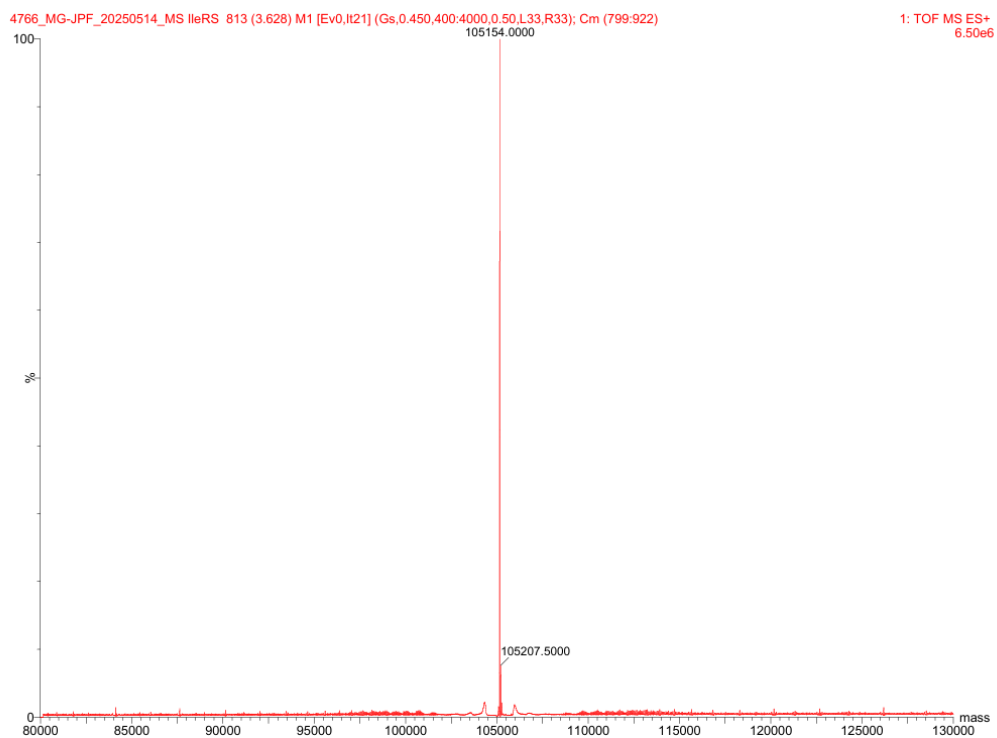
Figure S15: ESI-MS spectrum of SallerS1. MW = 105157.80 g/mol.
