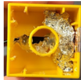
Figure 5.20.: Sensor brick with inserted jumper cable
