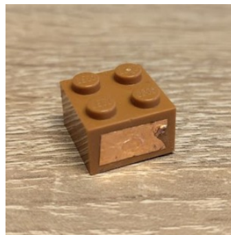
Figure 5.2.: Drilled horizontal vis-à-vis connection
