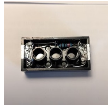
Figure 5.6.: Taped horizontal vis-à-vis connection
