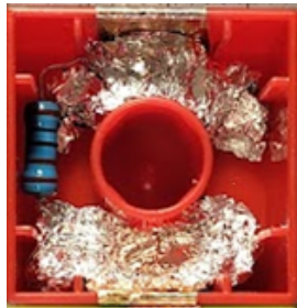
Figure 5.18.: Note brick containing a resistor
