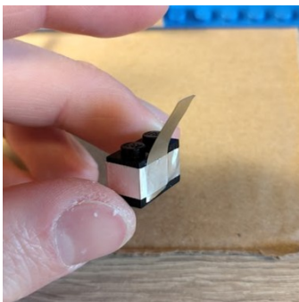
Figure 5.7.: Glued nickel-tape extension
