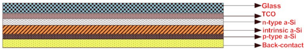
Fig. 2.14: Cross section of an a-Si cell.
