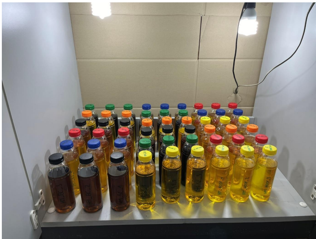
Fig. S1: Setup of storage study with 54 oil samples (black cumin, canola, sunflower, high-oleic sunflower, linseed and hempseed oil from three different suppliers in triplicates) in PET bottles stored at room temperature for 12 h under cold fluorescent light per day for six months.
