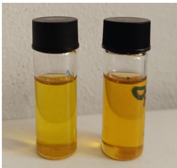
Fig. S2. Non-fortified (left) and PE-fortified (right) flaxseed oil after heating at 100°C for 10 h.
