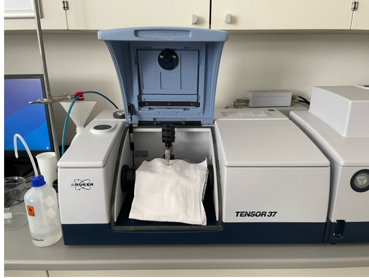
Figure 3.1.: The setup of an MIR spectroscopy measurement
