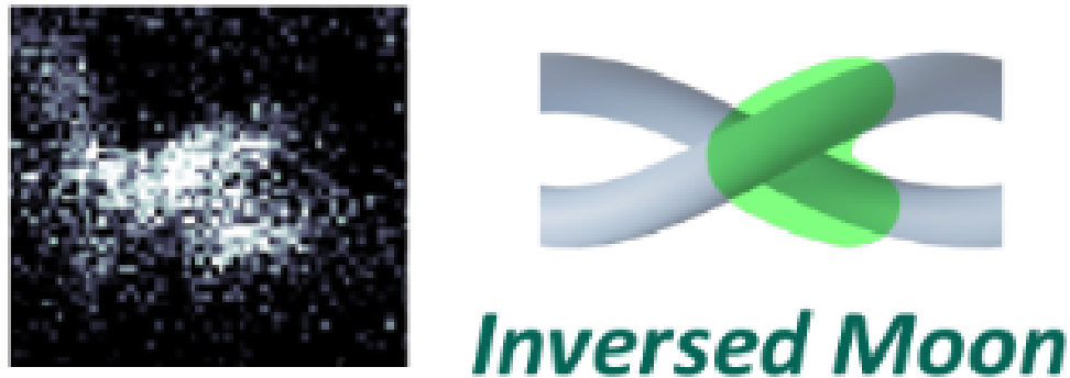
Figure 2.9.: Left: Experimental XMCD data post-processed with a Fourier Transform for the Structure F mode at 1.7 GHz. Right: 3D rendering of the structure from this perspective. Image courtesy of C. Donnelly and P. Morales Fernandez (Spin3D group, Max Planck Institute for Chemical Physics of Solids, Dresden).
