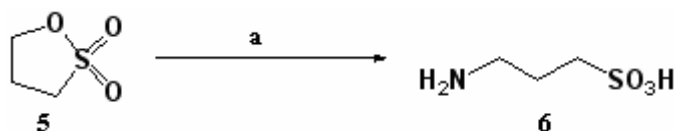
Fig. 4: Preparation of homotaurine (3-aminopropanesulfonic acid, 6 ) by ring opening of 1,3-propanesultone ( 5 ) Conditions: a: MeOH, NH 3 , -21°C to r.t, 18 hrs.
