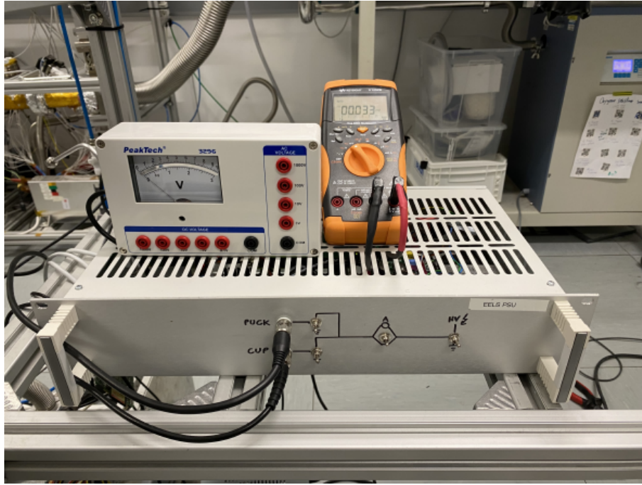
Figure 3.12: A photograph of the deceleration setup control unit. The front panel has switches to turn on the power supply, put the multimeter in the loop, and switch between the Faraday cup or the sample puck. An analog voltmeter that is used to readout the voltage supplied and a multimeter that is used to measure the beam current, are placed above the power supply unit.
