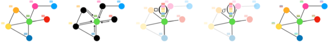
Figure 3.9: The message passing steps in order. First we have the input graph. Then the green node receives all of the neighbouring features, aggregates it through some invariant function. Then the message is transformed through the use of a neural network. Finally all the features in the graph get updated with their updates values. [BS24, p.23]
