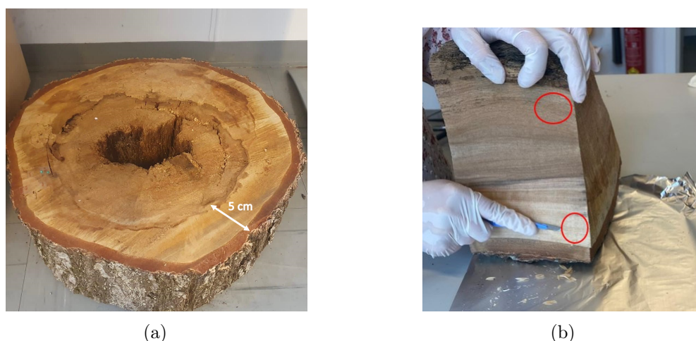
Figure 8.5: Birch trees from two different point of views, possibly contaminated with radioisotopes: (a) Tree disc as entire piece from above; (b) Section of tree disc prepared for sample examination, with red circles highlighting the selected rings.
