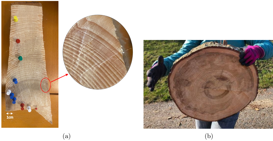
Figure 8.3: Coniferous trees: (a) Spruce.3 ( Picea abies ), estimated age: 105 years old; circled area points out the thinness of some tree rings; (b) Spruce.3 ( Picea abies ) as a whole piece, estimated age: 105 years old.
