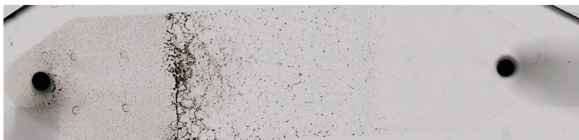
Picture 13. PDMS-based microfluidic reactor after the injection of 0.1 mM Fe(III) suspension at a flow rate of 1 ml/h; Showing a cluster of retained mineral from the inlet (left hole) of the reactor pore space to the front line of the pores (4x).
