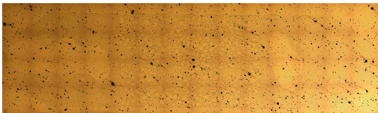
Picture 7. PDMS-based microfluidic device mixed with goethite powder (microscopic, stitched image; 4x)
