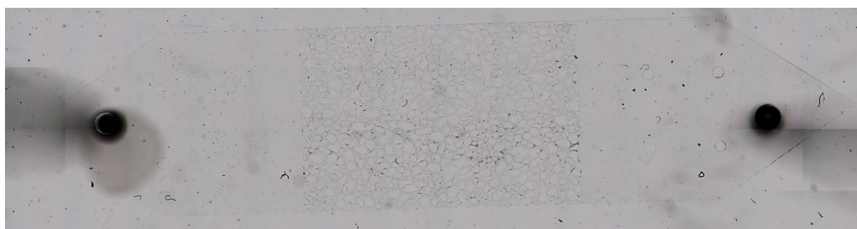
Picture 10. PDMS-based microfluidic reactor after the injection of 0.1 M \text{Cr}(\text{OH})_3 suspension at a flow rate of 1 ml/h and after flushing through 1 ml MilliQ water at 1ml/h; Showing retained mineral well distributed inside the reactor pore space (4x).
