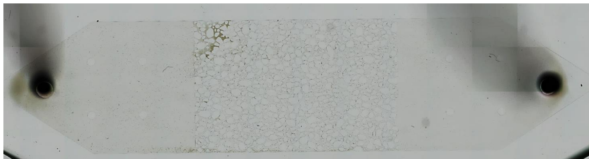
Picture 11. PDMS-based microfluidic reactor after the injection of 0.05 M Cr(OH) 3 suspension at a flow rate of 1 ml/h; Showing a cluster of retained mineral from the inlet (left hole) into the upper left corner of the reactor pore space (4x).
