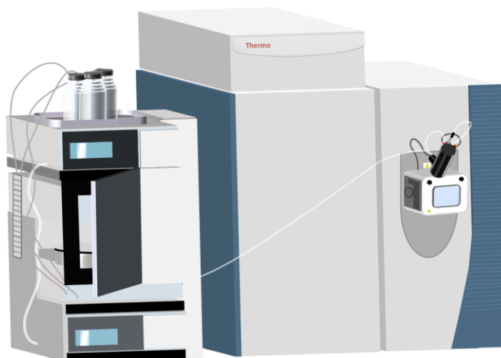
Figure 12: Vanquish Horizon UHPLC – Q Exactive HF Hybrid Quadrupole-Orbitrap – combination. Schematic drawing of the MS device used for the eicosanoid analysis of the sheep organ samples.
