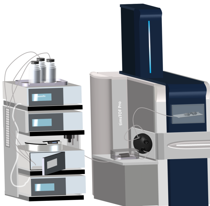
Figure 8: Schematic 3D-drawing of the setup of the LC-MS device used for the analysis of the proteome of the sheep organ-samples. Left: Ultimate 3000 nano-LC. Right: TIMS-TOF Pro (Bruker Daltonics).
