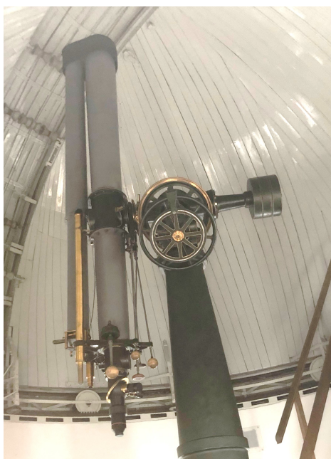
(a) The Kuffner Observatory's Large Refractor as seen from the side, with the hour angle scale visible (wheel in the centre of the mounting)
