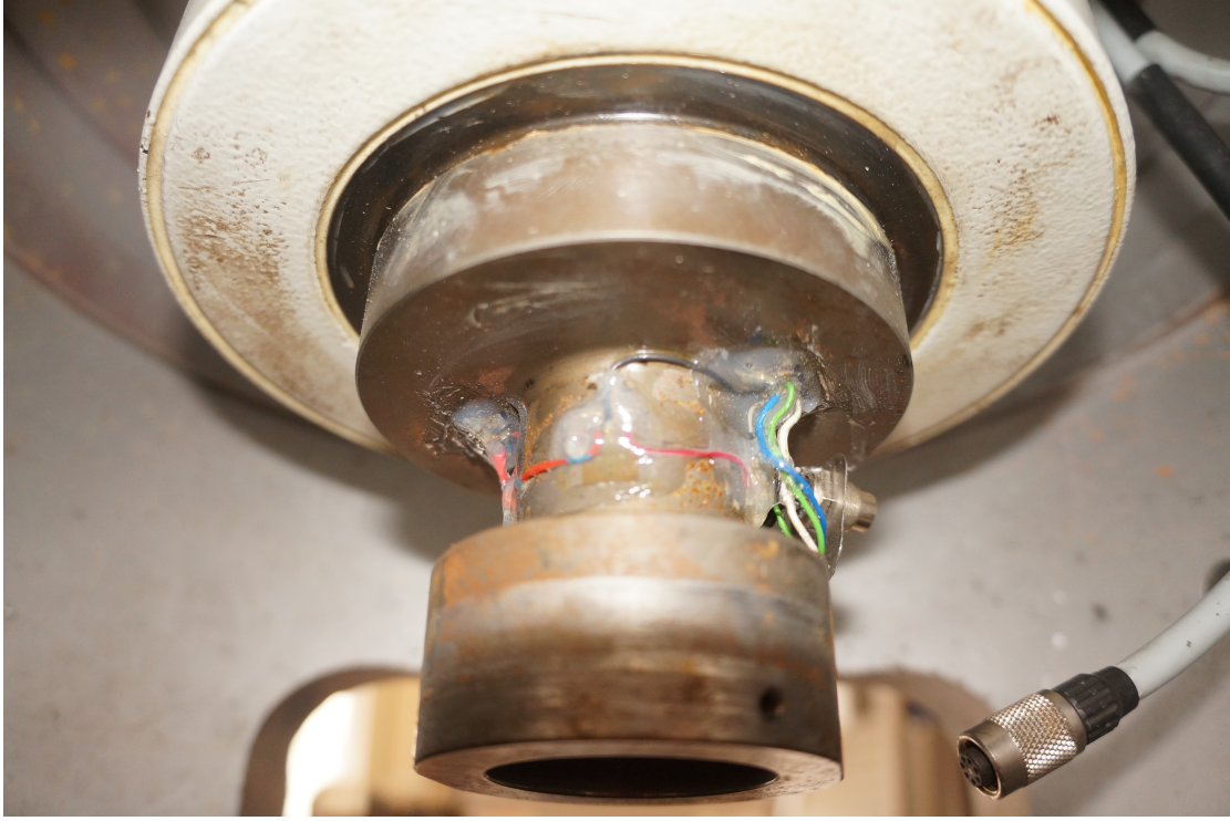
Figure 3.2: Photograph of the installed torque tool
