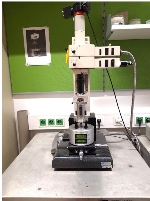
Figure 10: The AFM from Bruker used for sample analysis during the project
