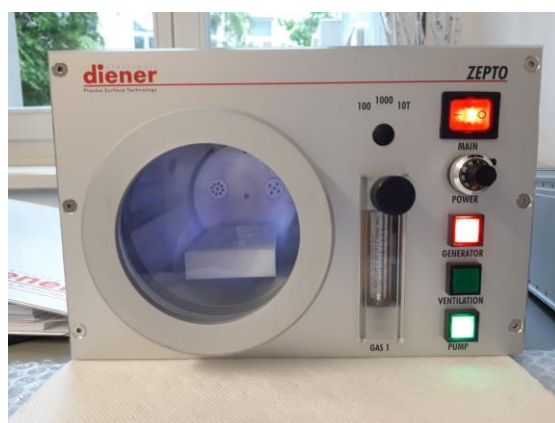
Figure 9: The plasma discharger used in the project
