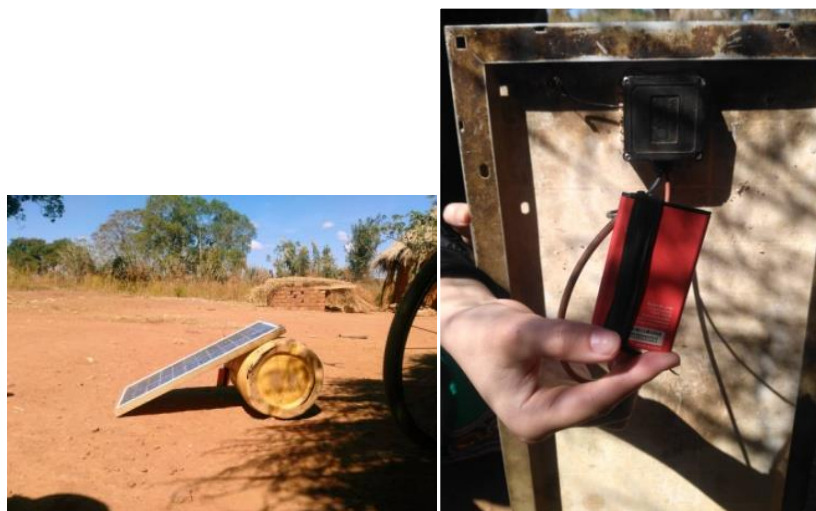
Figure 21: A Big Solar Panel Being Used to Charge a Basic Mobile Phone Battery
