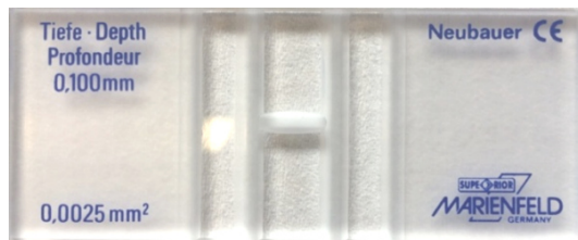
Figure 29: Hemocytometer/ Neubauer counting chamber produced by Marienfeld-Superior
