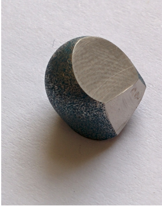
(a) Single crystalline sample of \text{Ni}_{0.90}\text{Pt}_{0.10} with surfaces cut in (110) orientation (top) and (100) orientation (side). The surface shows residues of aluminum oxide colored blue by nickel impurity.
