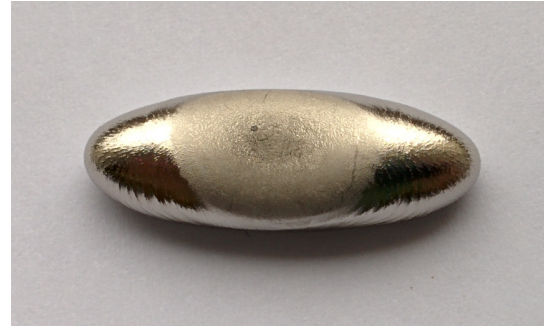
(b) A lump of a \text{Ni}_{75\text{at.}\%}\text{Pd}_{25\text{at.}\%} solid solution after cold boat melting.
