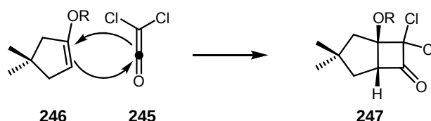
Scheme 45: [2+2]-cycloaddition of a cyclopentene derivative with dichloroketene
