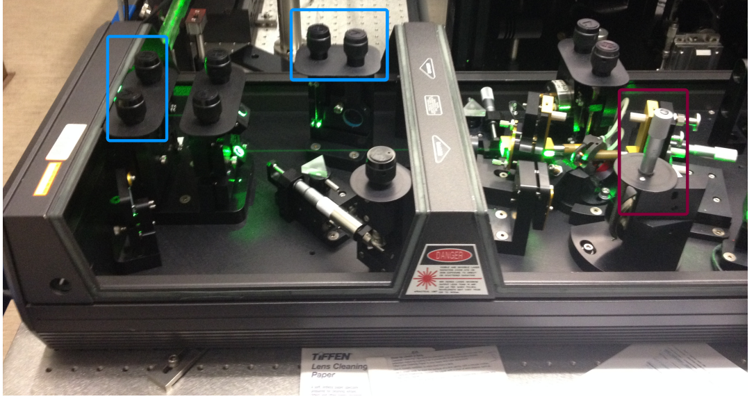
Figure 9: Part of the Mira900 without cover. The screws marked in blue should be used for aligning the Mira cavity. Marked in red is the screw that changes the wavelength of the emitted laser light which should be checked regularly.
