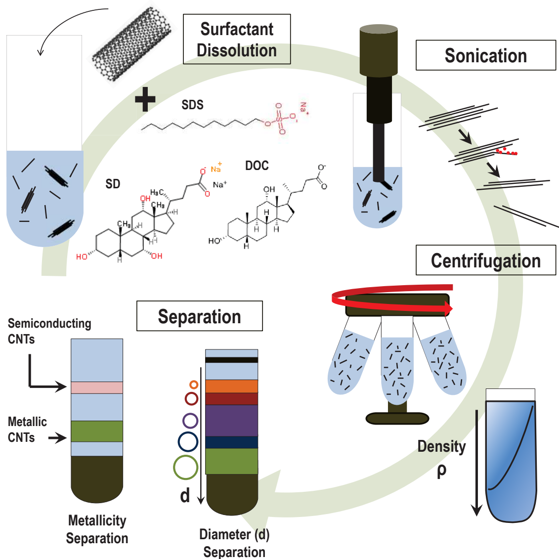
Figure 3.2. Density gradient ultracentrifugation (DGU) process. By using this method, it is possible to clean nanotubes as well as separate clean SWCNTs material according different characteristics. For example, by mixing the pristine SWNTs with surfactants, the metallic and semiconducting nanotubes can be separated from each other upon ultracentrifugation.
