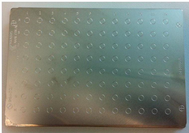
Figure 18 MALDI metal target used for the MS experiments. Samples were applied into the small ringed areas.
