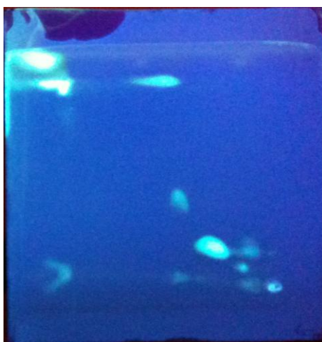
Figure 16 Example of a 2D HPTLC stained with primuline dye seen under UV light. Lower right was the starting point. For detail on the corresponding spots see chapter 4.1.1. Plate size 10x10cm.
