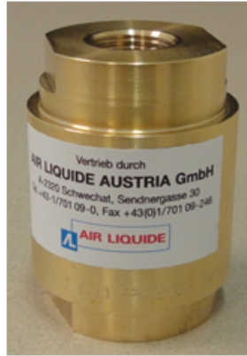
Figure 4.18: Picture of the mechanical safety valve.
