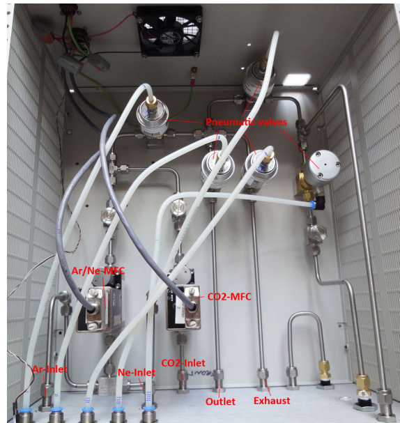
Figure 4.7: Top view of the "Mixing" module. In the bottom left corner, the two MFCs can be seen (left: Ar/Ne MFC, right: CO 2 MFC).
