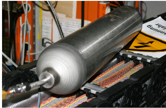
Figure 4.19: Picture of the GEM-TPC dummy volume used during the first tests of the closed gas system.
