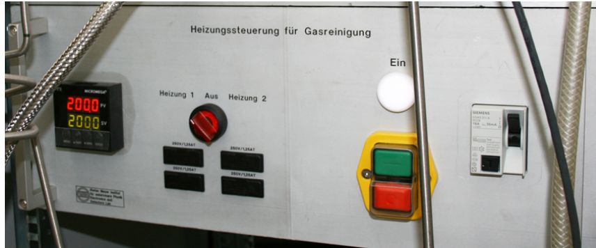
Figure 4.10: Picture of the heating module for the purification cartridge. The PID controller with a setpoint of 200°C can be seen on the left side.
