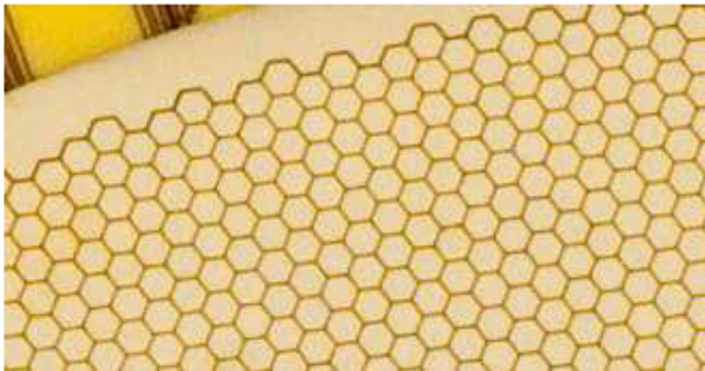
Figure 2.9: Picture of the pad plane of the GEM-TPC [13].
