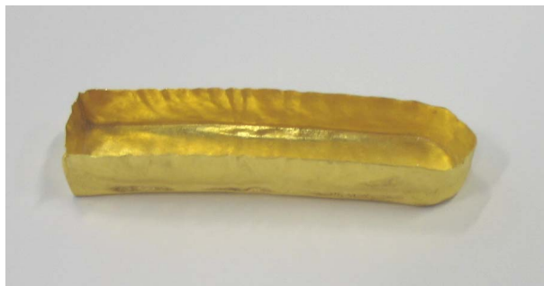
Fig.2.5: Gold crucible for calcination
