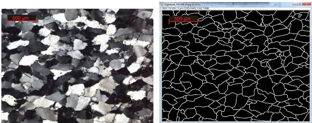
Figure 59: Quartzite used for shape preferred orientations measurement. Left: XPL image; Right: digitalized outlines of the grains.
