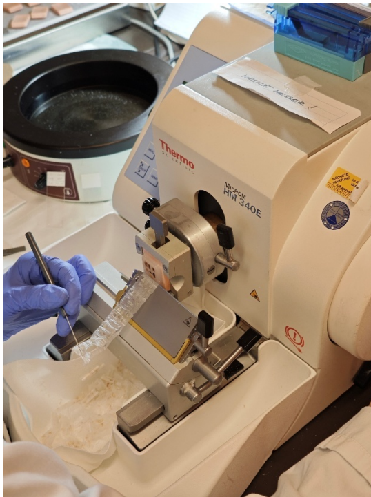
Supplementary Figure 3: Paraffin-embedded tissue section preparation using a microtome. Samples were cut in long bands at a thickness of 3 \mu m (A). Sections floating in a waterbath for stretching and being mounted on a glass slide (B).
