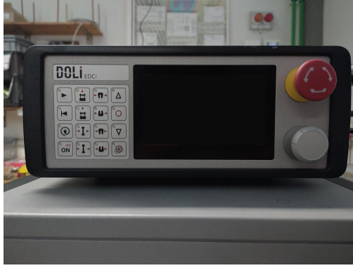
Figure 3.4.: Picture of the EDCi 22 controller for performing tensile test experiments.
