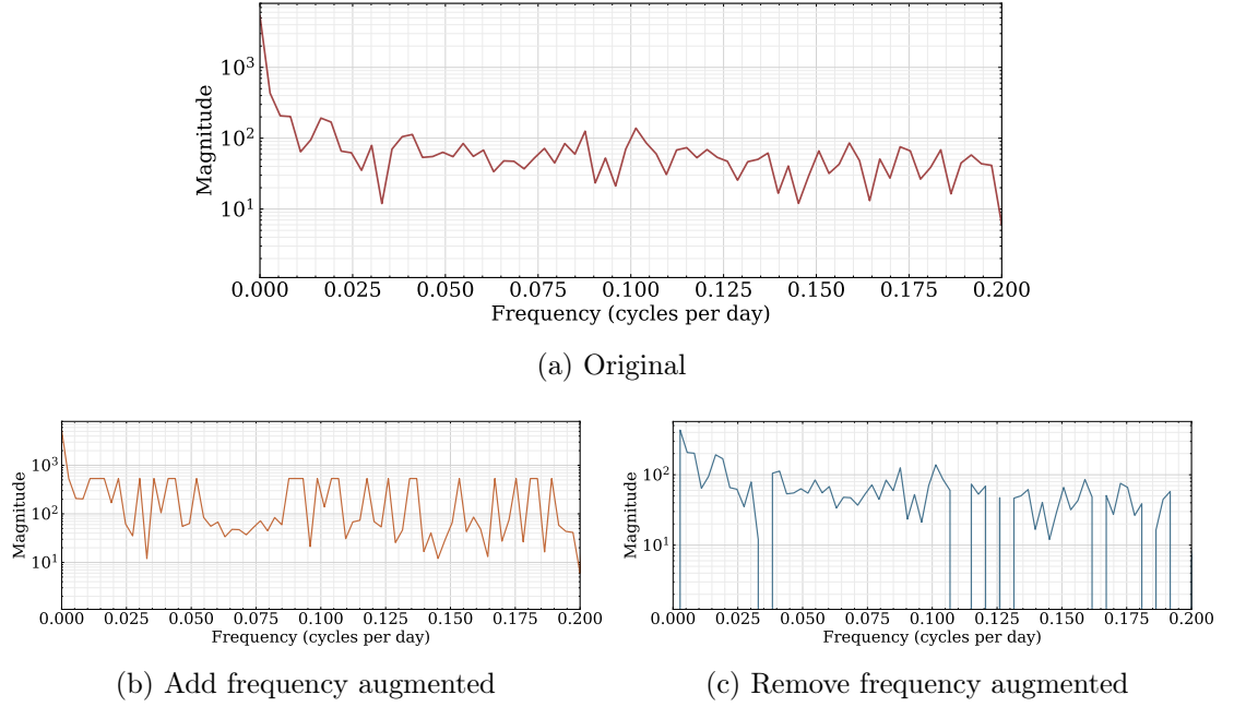
Figure 3.4.: Original and augmented views of a smart meter frequency-domain profile.
