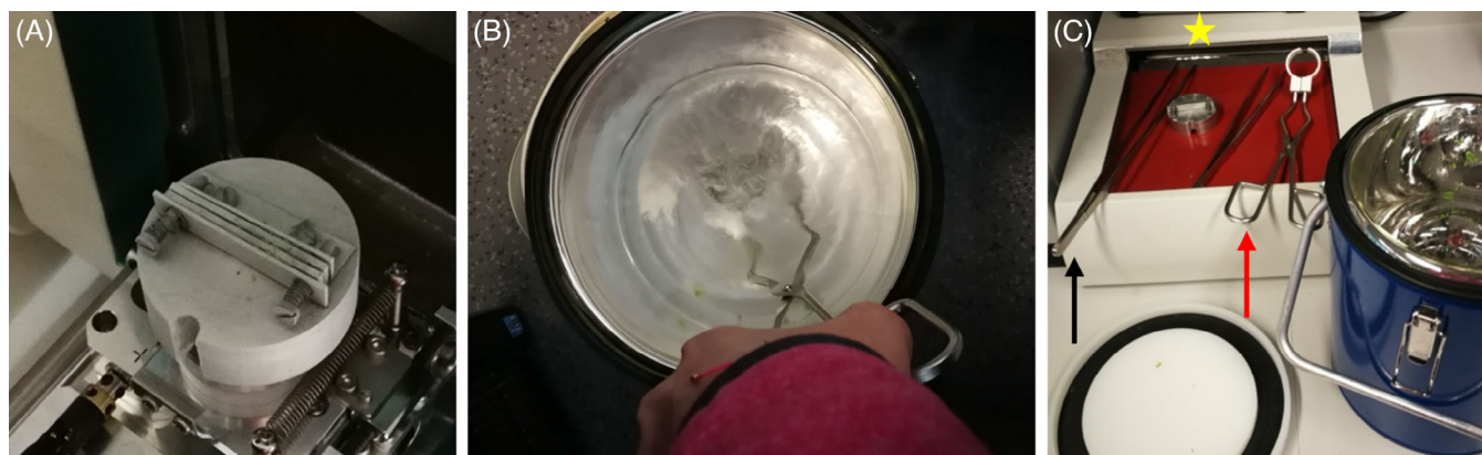
FIGURE 1 Sample preparation for EM: (A) custom-designed holder with three plunging spots; (B) the custom-built holder submerged in liquid nitrogen to freeze the mounted leaves; (C) the forceps used to immerse the leaf holder into liquid nitrogen (red arrow), and to hold the razor blade to cut the leaf while submerged in liquid nitrogen (black arrow), the heater to remove ice from the tools (yellow star).
