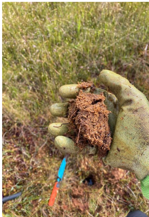
Figure B6: Peat degree of decomposition measurement according to von Post (1924) in Wörschach (own picture, 2025).
