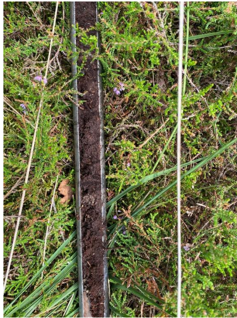
Figure B5: Peat thickness measurement with the Pürkhauer in Wörschach (own picture, 2025).
