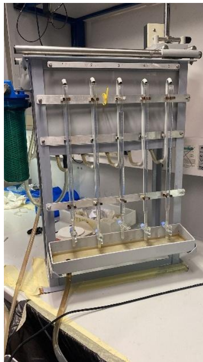
Figure 7: Royal Eijkelkamp device for permeability measurements (own picture, 2025)
