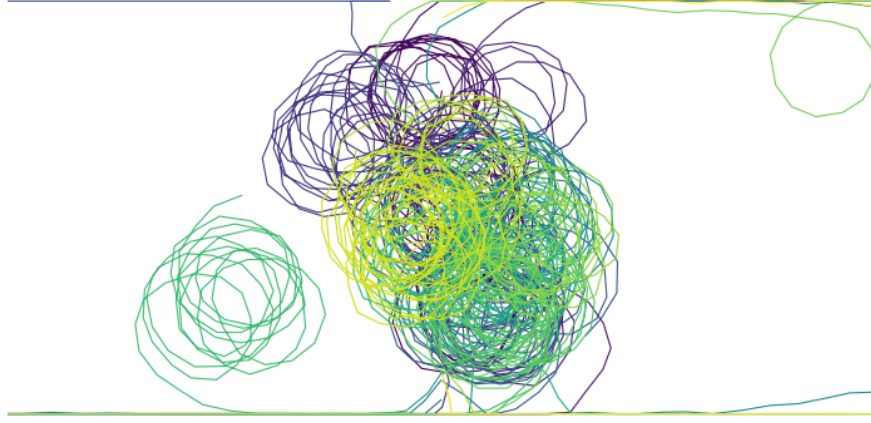
Figure 4.2: Typical simulated trajectories in a 40\ \mu\text{m} wide channel. For each simulation run, the swimming radius is kept constant. Here, it is set to R_0 = 10\ \mu\text{m} .
