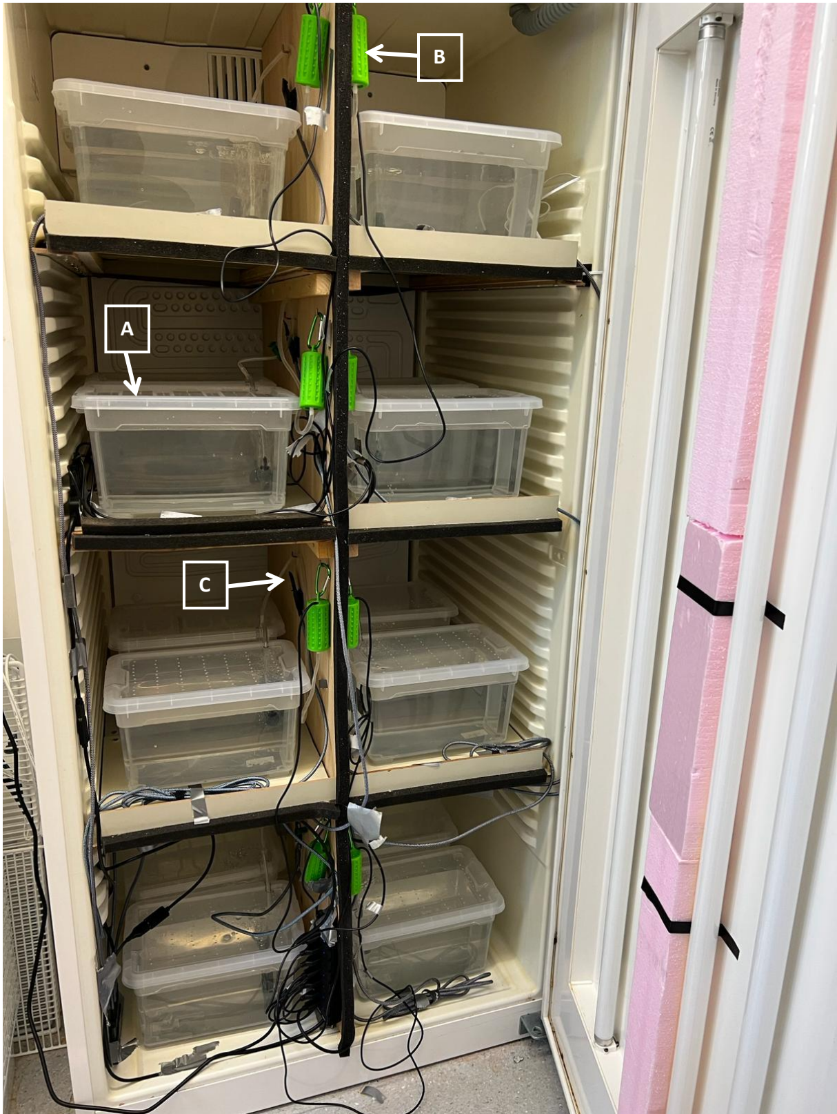
Figure 1: Experimental setup. The modified fridge contained 16 containers (A) in eight chambers. The temperature was set to 20°C, oxygen supply was ensured using air pumps (B) and associated air stones. During the day the light tubes attached to the door were on. At night small LED plates (C) were activated in the chambers of the experimental groups, the present LED plates in the chambers of the control groups were covered. When closed, the fridge was additionally secured with lashing straps.
