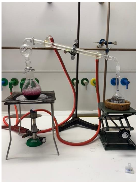
Figure 31: Distillation apparatus set up
