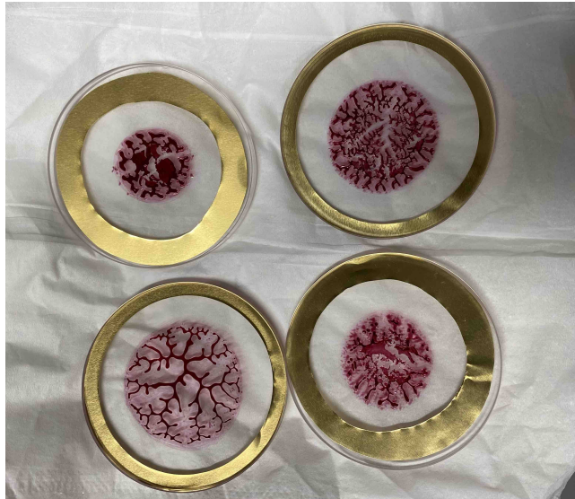
Figure A.2.: Fabrication failure from sample set S13, showing the retracted NDPC material between the two glass substrates.
