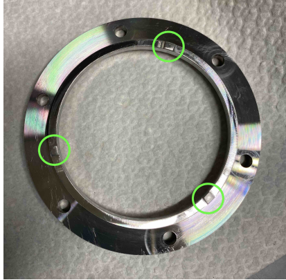
Figure 3.12.: Modified clamping ring used for sample set S15, incorporating three raised contact points for defined three point support (highlighted in green).
