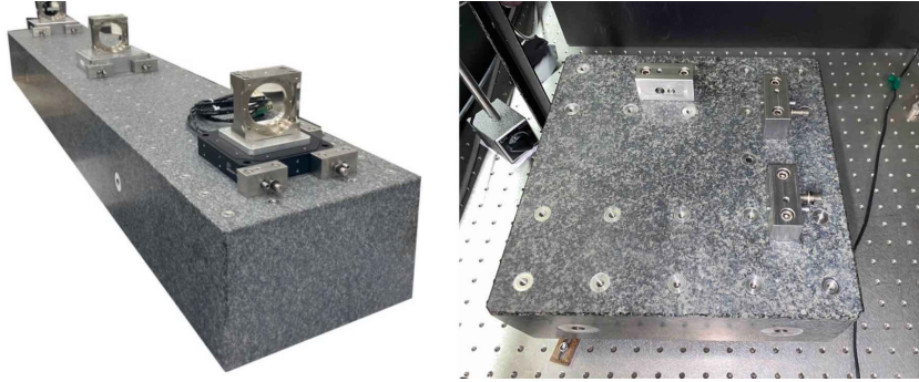
Figure 3.7.: Left panel: photograph of the granite bench used for the LLL interferometer setup (Image taken from Johann Fischer Aschaffenburg). Right panel: photograph of the small granite bench used for the recording of the gratings.
