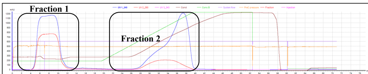
Figure 55 Cation exchange chromatography diagram from Run 3/8 of LPEI-PEG-OPSS Synthesis 1 in HEPES buffer. 5ml of crude polymer was injected and subjected to chromatographic separation by ÄKTA. Y-axis plots milli-Absorbance-Units and UV measurements are shown in colored lines (240nm blue, 280nm red and 343nm pink nm); blue line represents detected LPEI. Solid phase used was Macro-Prep High S Media and ÄKTA settings are described in Table 7; Fraction 2 subject to Centrifugal Filtration Purification;
