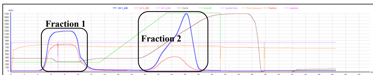
Figure 30 Cation exchange chromatography diagram from Run 1/8 of LPEI-PEG-OPSS Synthesis 2 in HEPES buffer. 5ml of crude polymer was injected and subjected to chromatographic separation by ÄKTA. Y-axis plots milli-Absorbance-Units and UV measurements are shown in colored lines (240nm blue, 280nm red and 343nm pink nm); blue line represents detected LPEI. Solid phase used was Macro-Prep High S Media and ÄKTA settings are described in Table 11; Fraction 2 subject to Centrifugal Filtration Purification ; please note that the diagrams of the remaining runs (2-4) are listed in the Appendix
