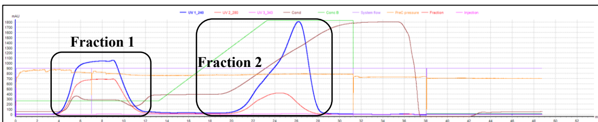
Figure 62 Cation exchange chromatography diagram from Run 4/8 of LPEI-PEG-OPSS Synthesis 2 in HEPES buffer. 5ml of crude polymer was injected and subjected to chromatographic separation by ÄKTA. Y-axis plots milli-Absorbance-Units and UV measurements are shown in colored lines (240nm blue, 280nm red and 343nm pink nm); blue line represents detected LPEI. Solid phase used was Macro-Prep High S Media and ÄKTA settings are described in Table 11 ; Fraction 2 subject to Centrifugal Filtration Purification
