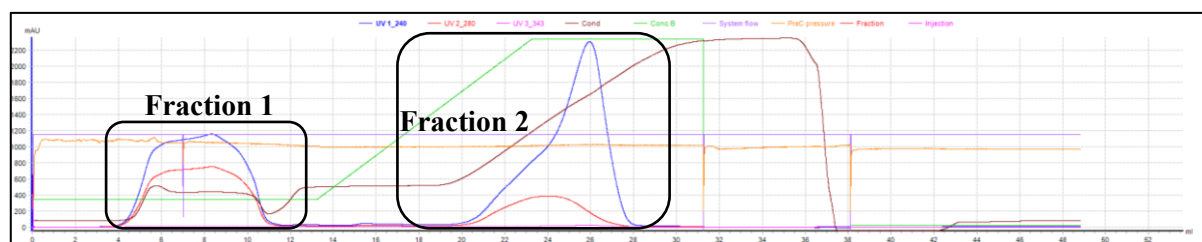
Figure 58 Cation exchange chromatography diagram from Run 7/8 of LPEI-PEG-OPSS Synthesis 1 in HEPES buffer. 5ml of crude polymer was injected and subjected to chromatographic separation by ÄKTA. Y-axis plots milli-Absorbance-Units and UV measurements are shown in colored lines (240nm blue, 280nm red and 343nm pink nm); blue line represents detected LPEI. Solid phase used was Macro-Prep High S Media and ÄKTA settings are described in Table 11 ; Fraction 2 subject to Dialysis Purification;
