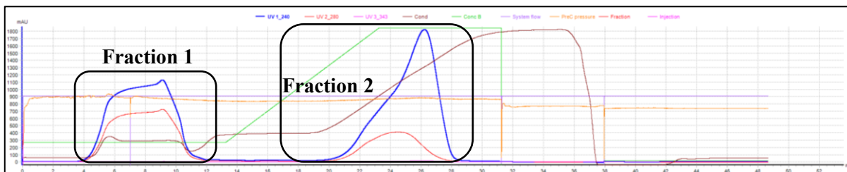
Figure 63 Cation exchange chromatography diagram from Run 6/8 of LPEI-PEG-OPSS Synthesis 2 in HEPES buffer. 5ml of crude polymer was injected and subjected to chromatographic separation by ÄKTA. Y-axis plots milli-Absorbance-Units and UV measurements are shown in colored lines (240nm blue, 280nm red and 343nm pink nm); blue line represents detected LPEI. Solid phase used was Macro-Prep High S Media and ÄKTA settings are described in Table 11 ; Fraction 2 subject to Dialysis Purification
