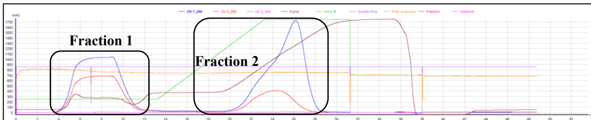
Figure 61 Cation exchange chromatography diagram from Run 3/8 of LPEI-PEG-OPSS Synthesis 2 in HEPES buffer. 5ml of crude polymer was injected and subjected to chromatographic separation by ÄKTA. Y-axis plots milli-Absorbance-Units and UV measurements are shown in colored lines (240nm blue, 280nm red and 343nm pink nm); blue line represents detected LPEI. Solid phase used was Macro-Prep High S Media and ÄKTA settings are described in Table 11 ; Fraction 2 subject to Centrifugal Filtration Purification
