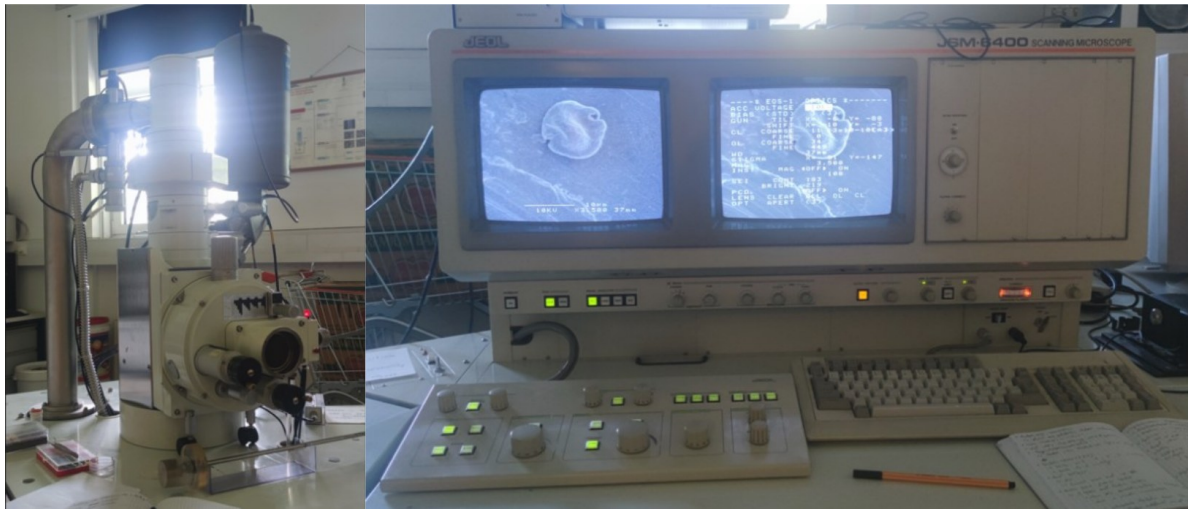
Figure 12. Electron Microscope (JSM-6400 Scanning Microscope) used and its associated monitors.
