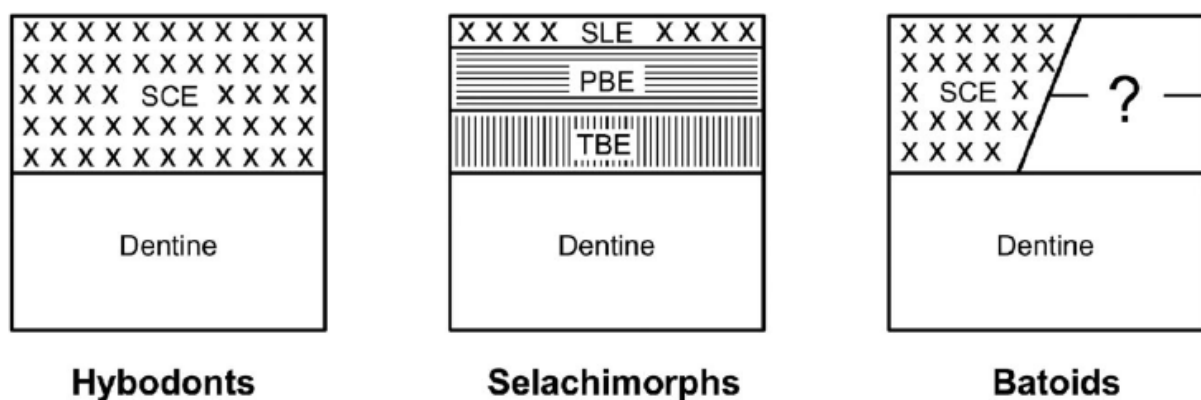
Figure 7. Schematic organization of the enameloid layers in hybodonts, selachimorphs and batoids (after Enault et al. (2013)).
