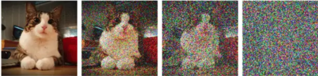
Figure 2.3.: Illustration of diffusion in generative modeling: the gradual addition of noise to transform structured data into pure noise. Source: NVIDIA Developer Blog
