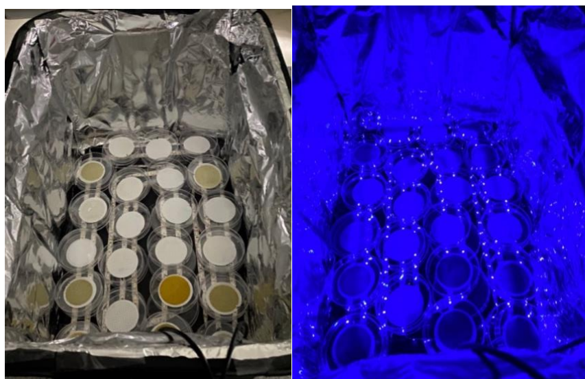
Figure 11: Left, membrane filters after filtration of samples and treatment with PMA before incubation; Right: The same samples incubated with the light source turned on.
