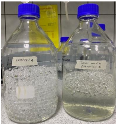
Figure 12: Retained filtrate after 24-hour incubation with TCT Target Beads for two different treatment steps (Control and Dual Media Filtration). These treatment steps are expected to differ greatly in DNA concentration, resulting in different final volumes.
