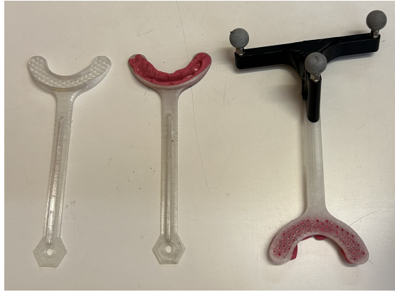
Figure 3.3.: Maxilla mouthpiece tracker mounts. Unused 3D printed maxilla mount (left), used maxilla mount with dentistry putty (center), and maxilla mouthpiece mount with neuronavigation tracker attached (right).
