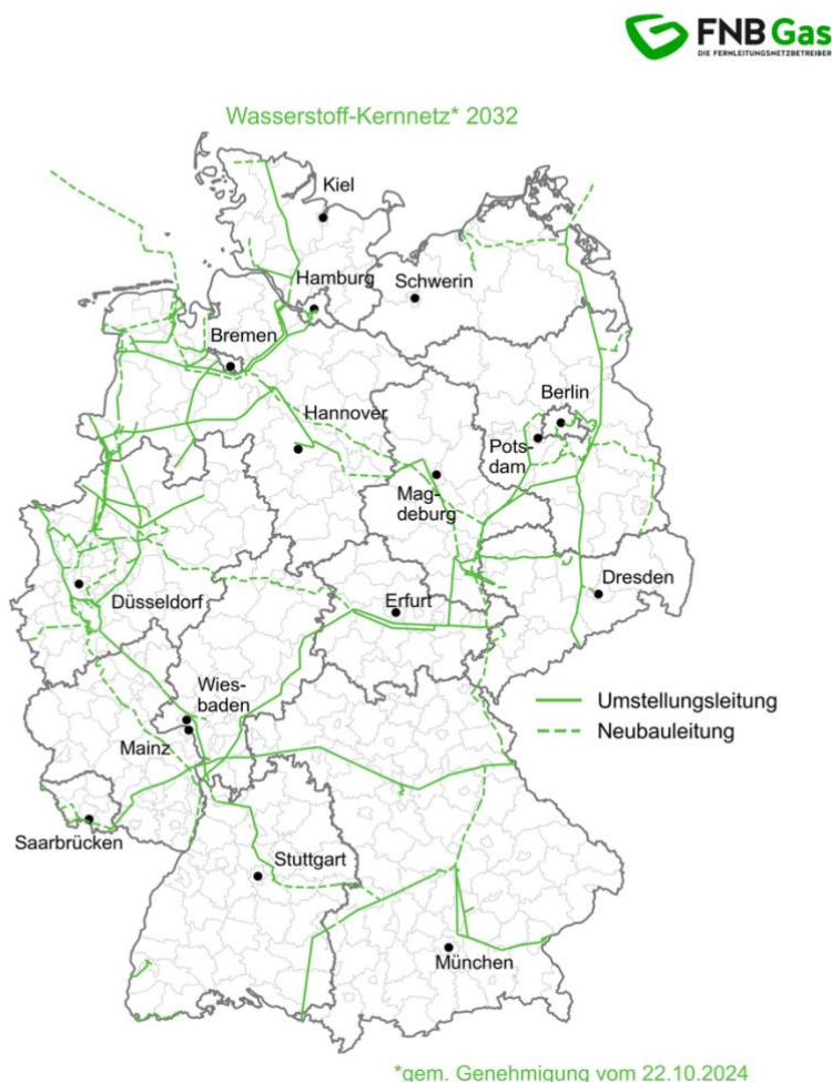
Figure 1 - Hydrogen core network (Source: FNB Gas, n.d.)
