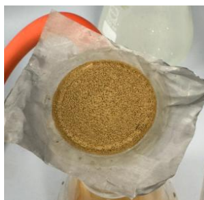
Figure 4.3: Rinse Fe(II) solution with 25 µm mesh, method OMR – DC (sample 10g – 5M soil)
