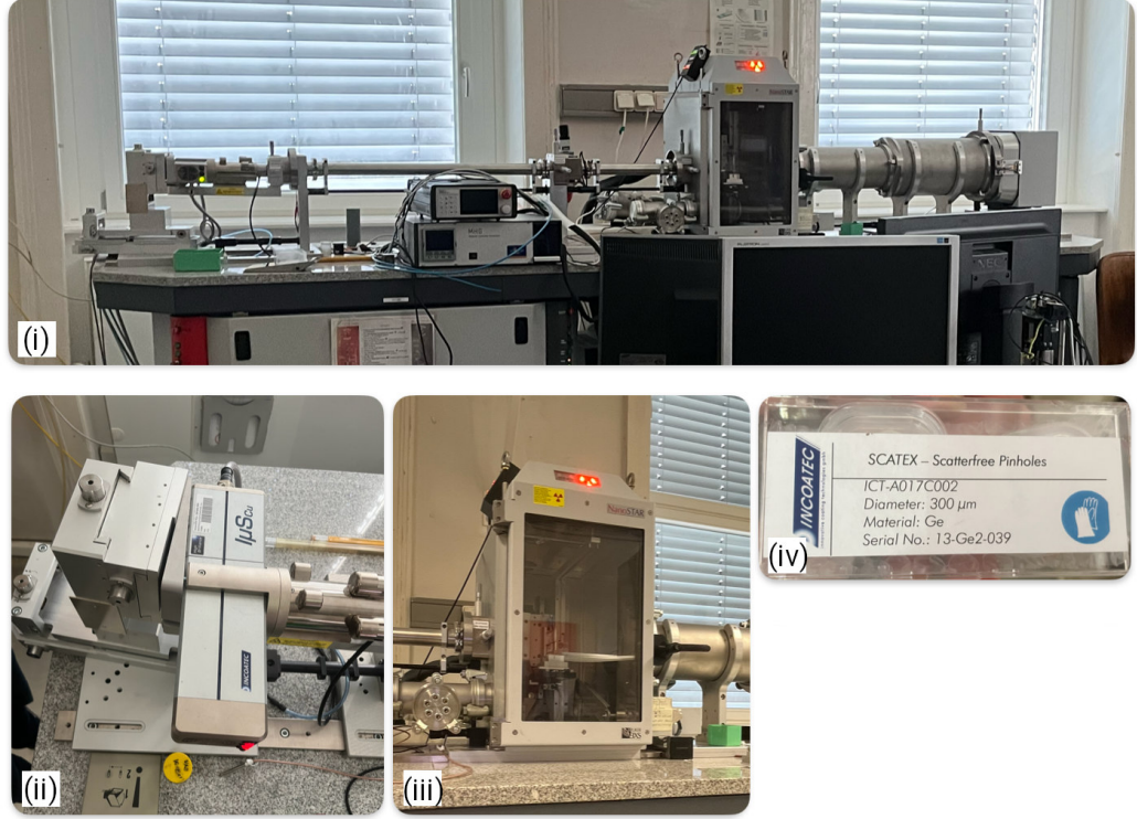
Figure 3.1.: Components of the Bruker AXS Nanostar Small Angle X-ray Scattering setup. (i) General view of the instrument. (ii) X-ray tube and beam collimation stage. (iii) Sample vacuum chamber inside the protective housing. (iv) Scatter-free pinholes (diameter 300 \mu\text{m} , Ge) applied for beam shaping and reduction of parasitic scattering.
