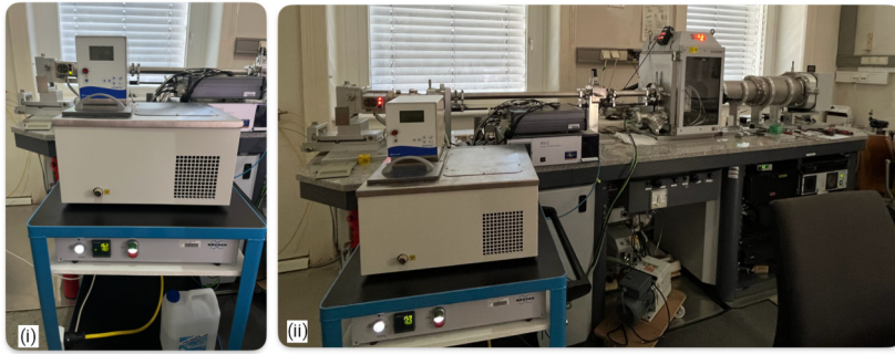
Figure 3.3.: Temperature control unit coupled to the Bruker AXS Nanostar SAXS setup. (i) Fisher Scientific Cooling device with Bruker control panel. (ii) Integration of the cooling unit with the SAXS instrument for performing temperature-dependent measurements.
