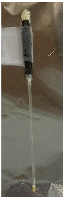
Figure A.1.: HFIP sample with white deposits have formed at the top of the capillary near the closure
