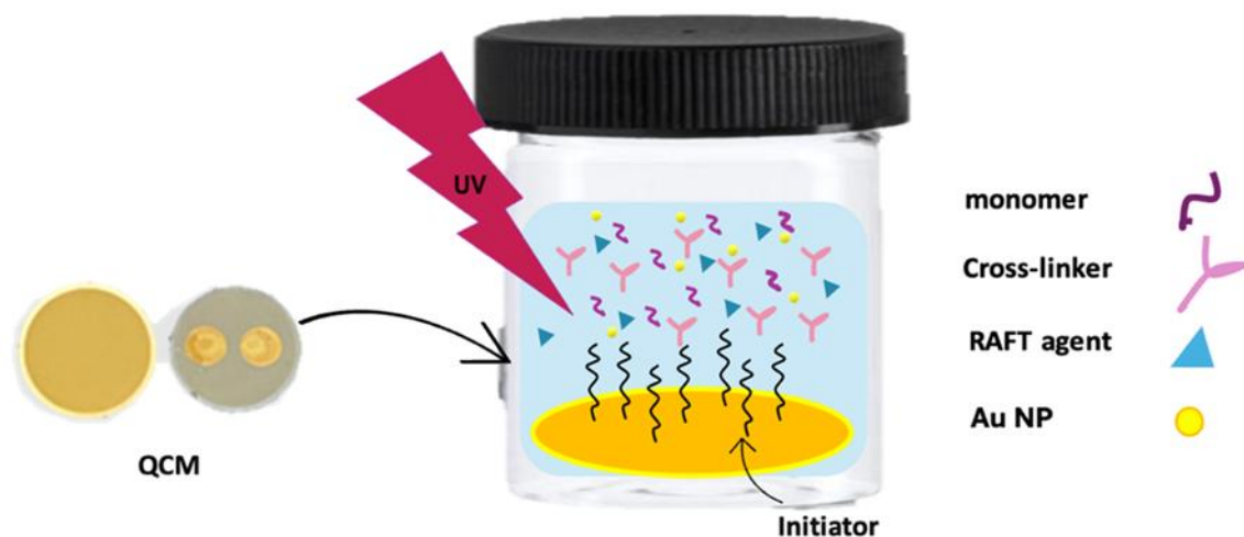
Figure 54: Schematic of in-situ polymerization of MIP.
