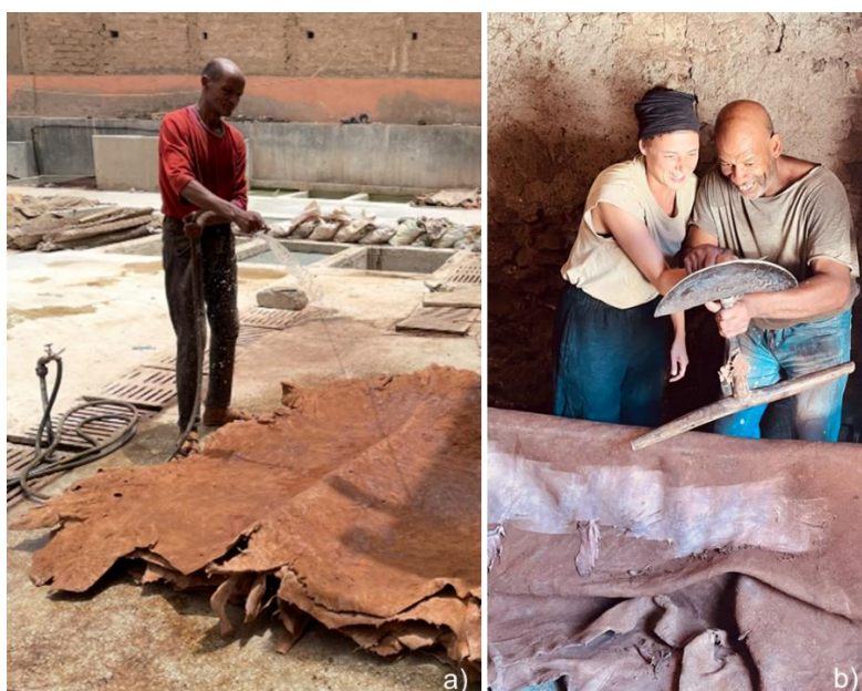
Fig. 39: a) A co-worker is preparing the cattle skin for the sedriya by sprinkling water on it (Photo: V. Immervoll, Marrakech, July 2024); b) A specialized co-worker is explaining the sedriya to the researcher (Photo: H. Rafik, Marrakech, September 2023)
