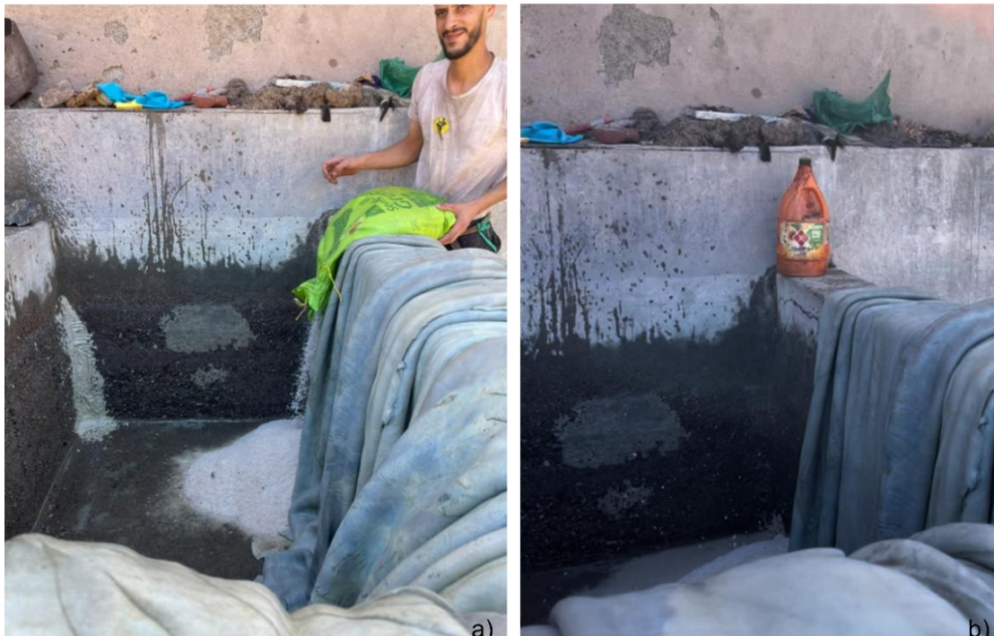
Fig. 34: a) An apprentice is giving salt into the high-above basin for the salt bath; b) The orange plastic bottle contains the acid for the salt bath (Photos: V. Immervoll, Marrakech, February 2024)
