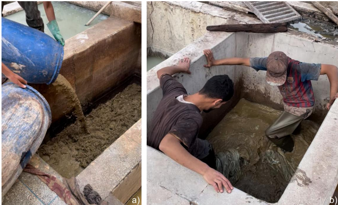
Fig. 33: a) Preparation of a bating solution by pouring pigeon droppings mixed with water into a rectangular vat; b) foot massage for sheep skins carried out by two apprentices (Photos: V. Immervoll, Marrakech, February 2024)
