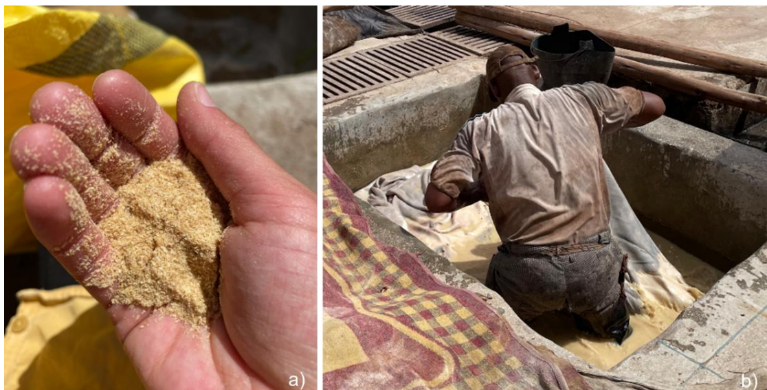
Fig. 35: a) Sample of the wheat bran used for bran drenching; b) A co-worker flips a cattle skin upside down inside a rectangular vat (Photos: V. Immervoll, Marrakech, March 2024)
