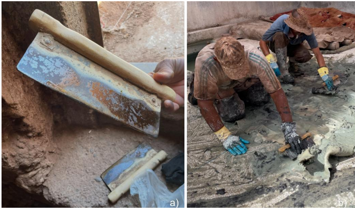
Fig. 31: a) The “ assawa hafia ” tool used for dehairing which becomes the “ assawa madeya ” for fleshing after sharpening on the whetstone (Photo: V. Immervoll, Marrakech, September 2023); b) Two co-workers carrying out the second dehairing of a cattle skin (Photo: V. Immervoll, Marrakech, March 2024)
