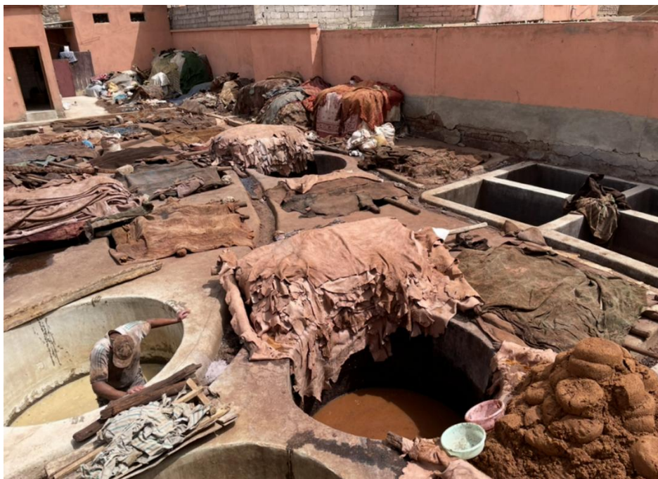
Fig. 37: Area with partly covered round vats for tanning; visible are cattle skins outside for breathing and the tanning agent which is spread layer by layer on the skins when given back to the vat (Photo: V. Immervoll, Marrakech, July 2024)
