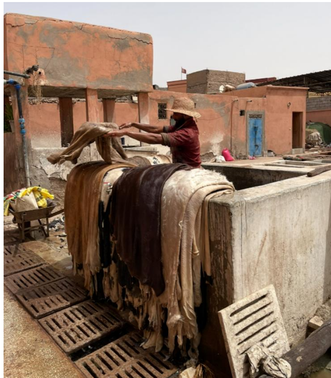
Fig. 27: A m'ellem placing calf raw skins over the edge of the merkel (Photo: V. Immervoll, Marrakech, February 2024)
