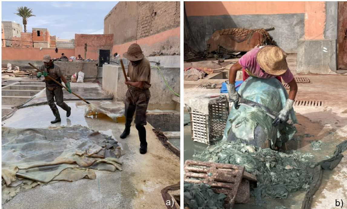
Fig. 32: a) A m'ellem and his co-worker putting out a cattle skin with the l-khtaff after the third liming bath; b) The s'kkim method carried out by a ṣān' (Photos: V. Immervoll, Marrakech, February 2024)
