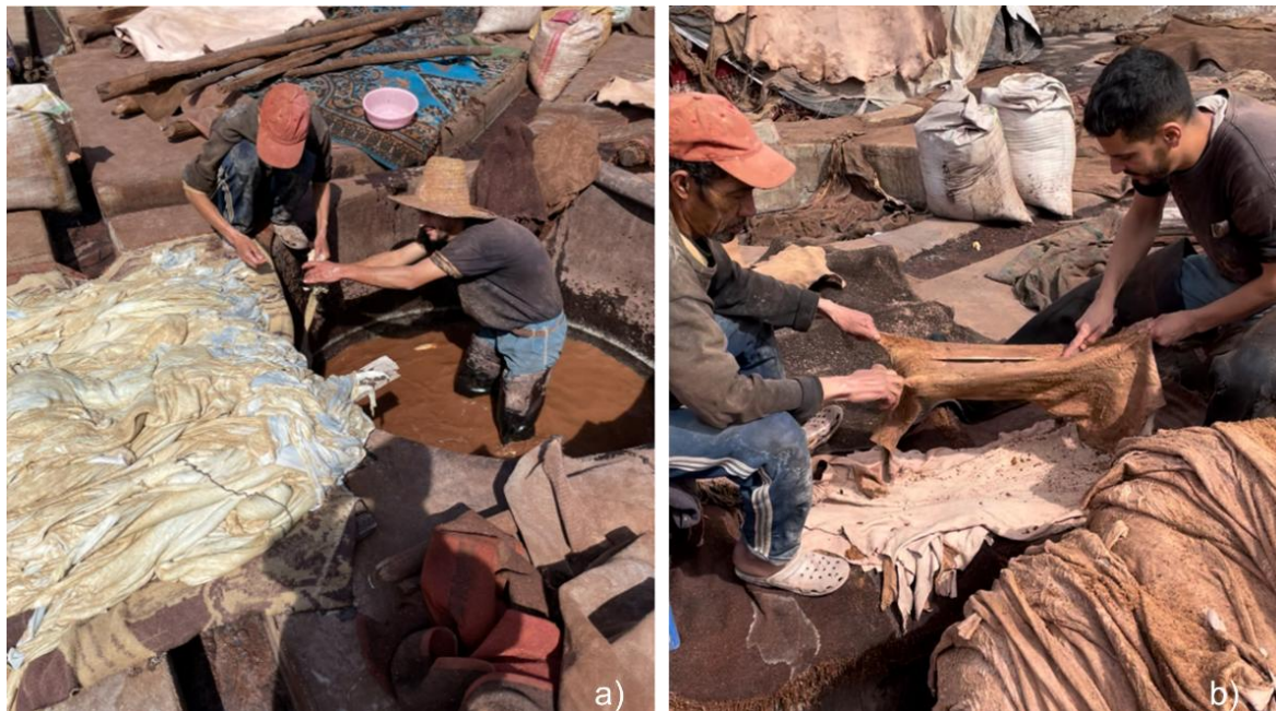
Fig. 36: a) An experienced co-worker (on the left with the red cap) and an apprentice putting sheep skins into a round vat for pre-tanning; b) Same tanners carrying out the shqān , starting with the first cut along the belly (Photos: V. Immervoll, Marrakech, March 2024)
