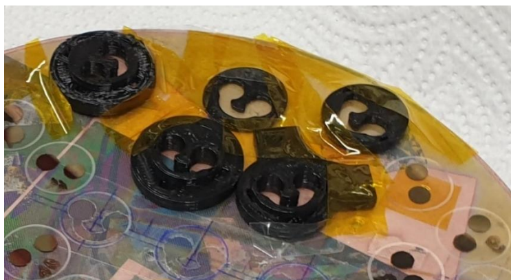
Figure 40: QCM masks fixed with tape on PVD plate.
