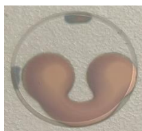
Figure 41: QCM that resulted from one of the thicker masks from the first batch.
