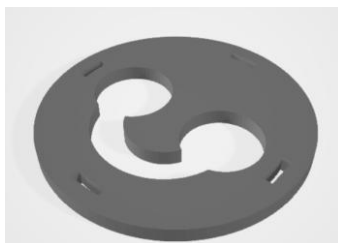
Figure 33:(Design 1.1) QCM mask design first batch. A fully flat mask with slits
