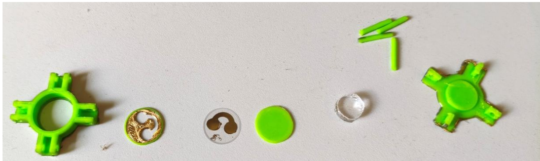
Figure 72: A photo of how all the final mask assembly looked. (after PVD)
