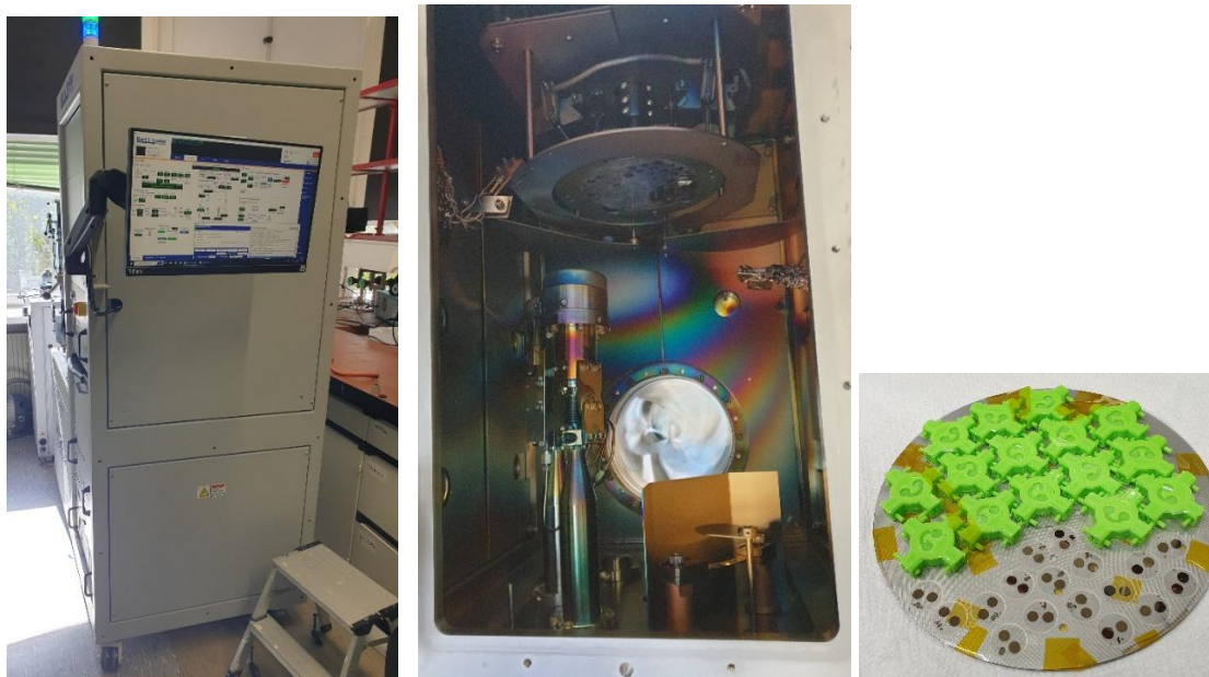
Figure 25: PVD machine (left) outside of machine (middle) sample chamber (right) PVD sample plate with QCMs before deposition
