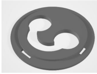
Figure 34: (Design 1.2) QCM mask design first batch. A mask with an elevated patch for easier grip
