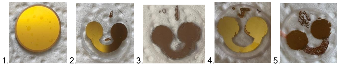
Figure 74: QCMs resulting from different manufacturing methods. 1. Fully coated QCM, 2. 3D-printed mask partially coated QCM, 3. Screen printed partially coated QCM, 4. Parasol foil mask partially covered QCM, 5. Parasol foil mask and screen-printed bridge partially covered QCM.
