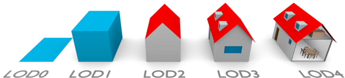
Abbildung 9: Levels of Detail in CityGML Quelle: BILJECKI et al. 2016
