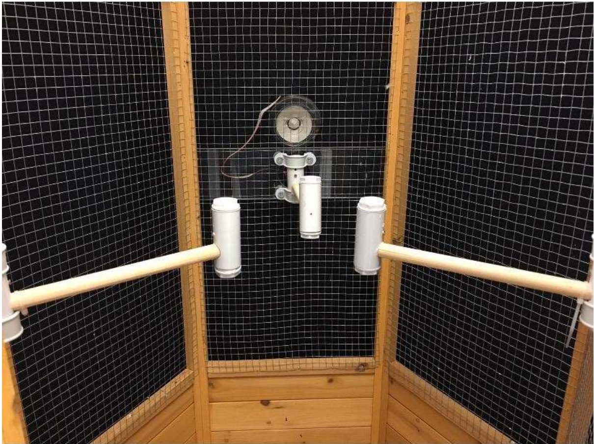
Figure 12.: Picture of the Inside view of the Testing Apparatus. The perches each are equipped with an infrared emitter and sensor, in front of a speaker.
