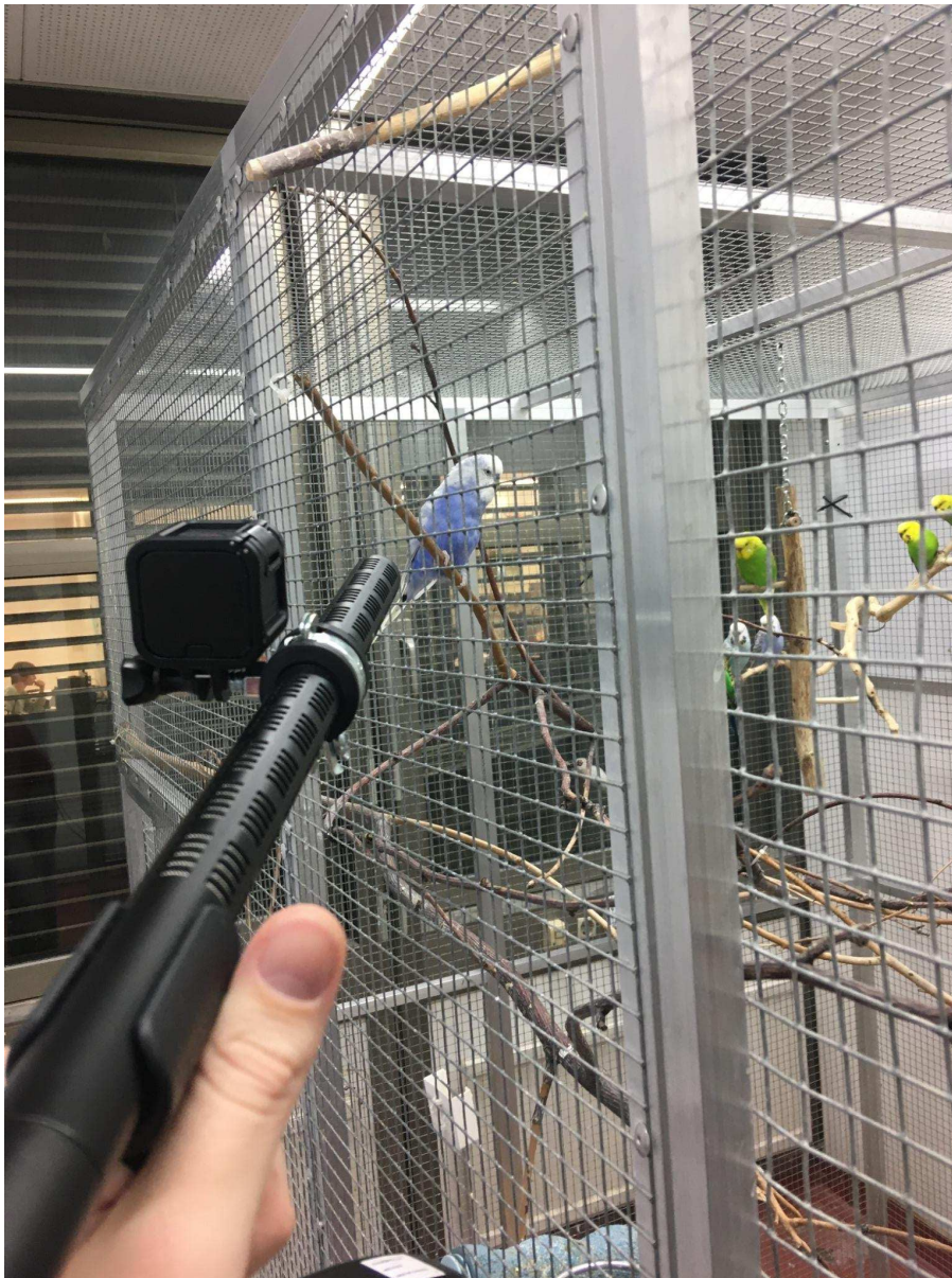
Figure 10.: Picture of how the Sound files were recorded before the experiments. The songs were recorded with a Sennheiser directional shotgun microphone. A GoPro Hero 4 was mounted on the microphone to identify the individuals vocalising (similar to Mann et al. 2021)
