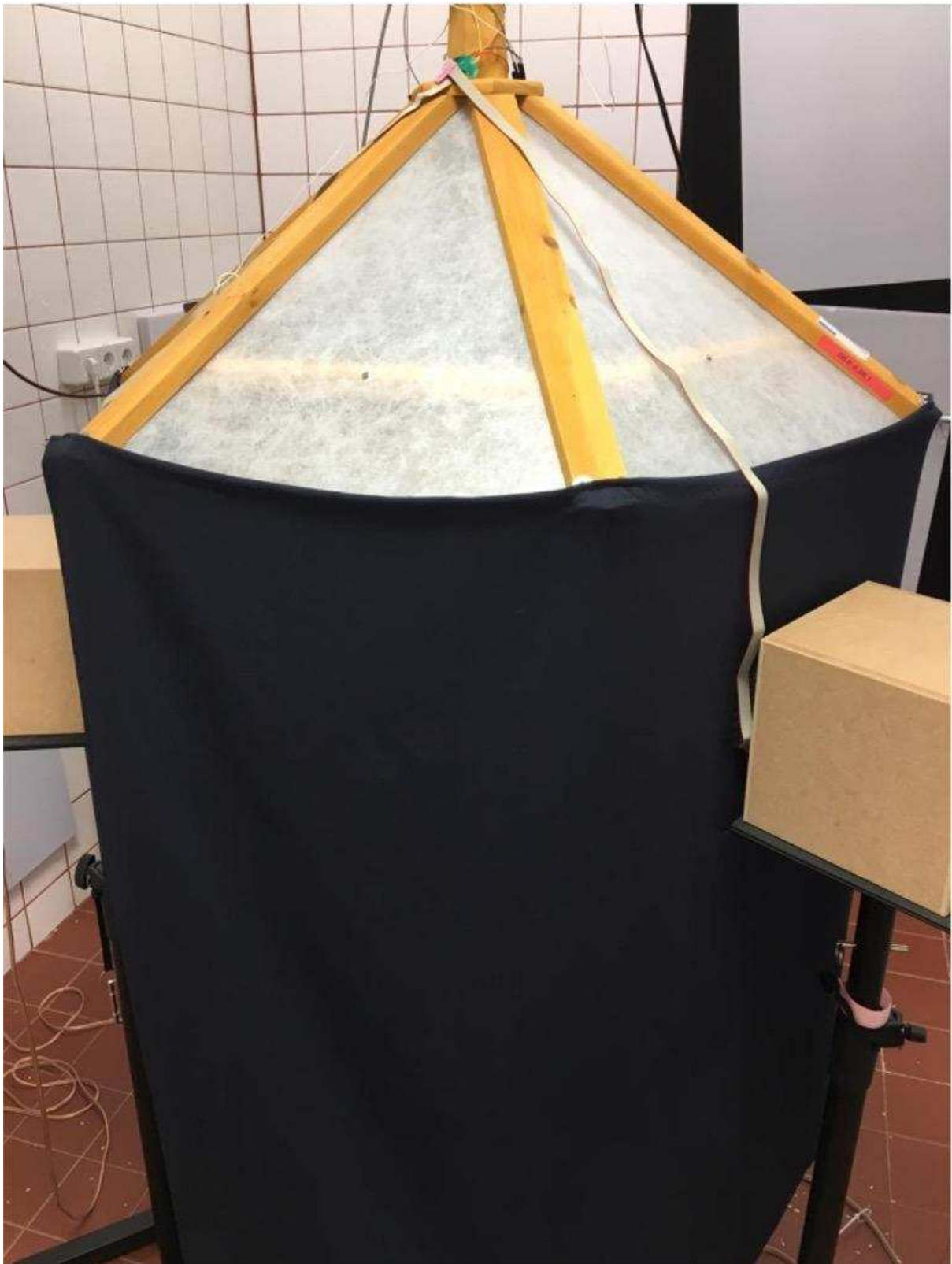
Figure 11.: Picture of the hexagonal testing apparatus at the Animal care facility (Universität Wien Althanstraße), surrounded by the three speakers.
