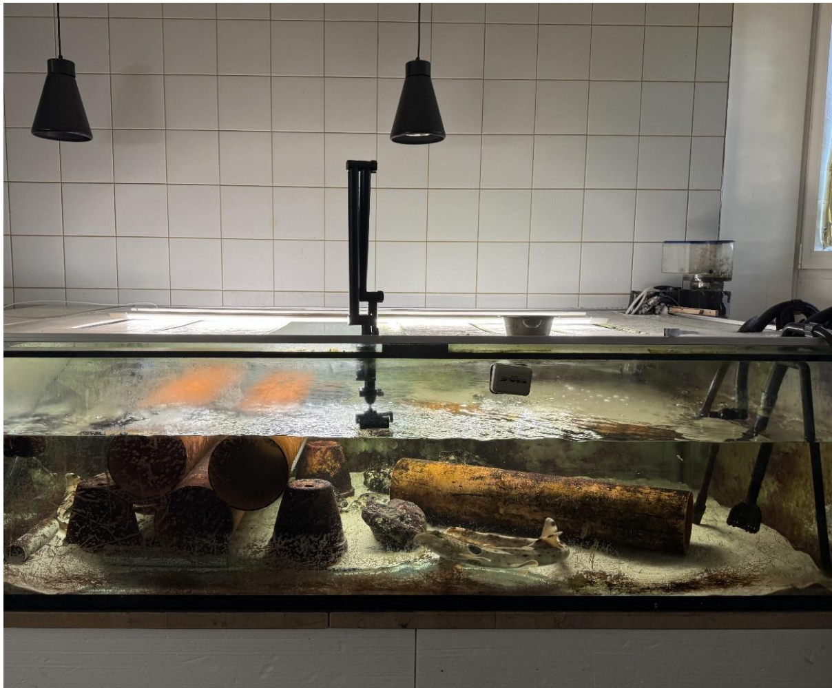
Figure 3. Setup of video recording equipment using a clamp tripod mounted on the aquarium.
