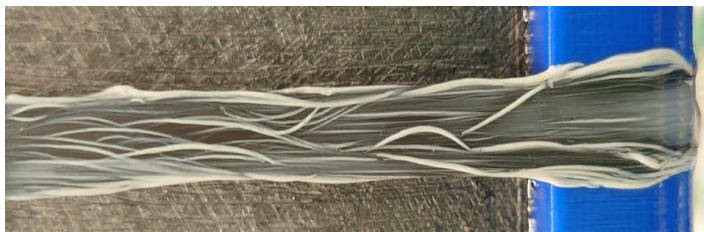
Figure 21: Macroscopic electrophoretic deposition of LDH from 72 vol% ethanolic suspension.
